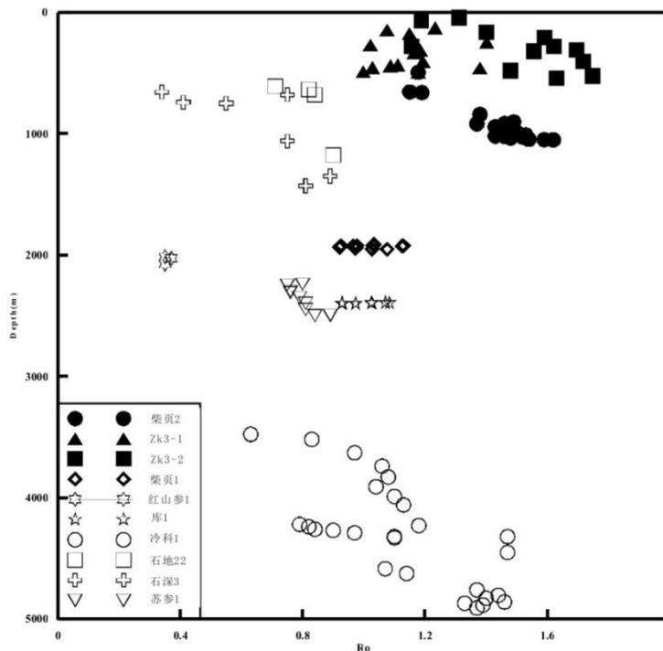
Fig. 5 Ro measurement distribution with depth from the studied wells in the Qaidam Basin
