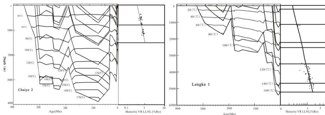
**Fig. 6** The modeled results of burial, thermal, and hydrocarbon generation history of Well Chaiye 2 and Lengke 1 in the eastern Qaidam basin. "•" means measured vitrinite reflectance and the solid line means modeled values in the right chart
