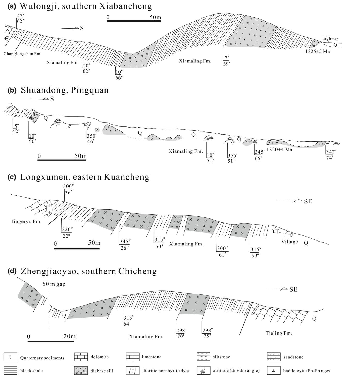
**Fig. 14.5** Cross sections showing the diabase sills emplaced into the Xiamaling Formation in the Yanliao rift (aulacogen) in the northern NCC (modified after Zhang et al. 2009, 2012c)
